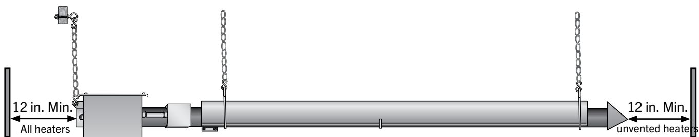
Figure 3.25 • Minimum End Clearances
