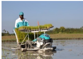
Fig. 2: www.kubota.global.net/english shows a Japanese-type walk behind transplanter
