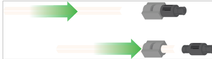
Removal of a standoff from a Mini Standoff Connector
