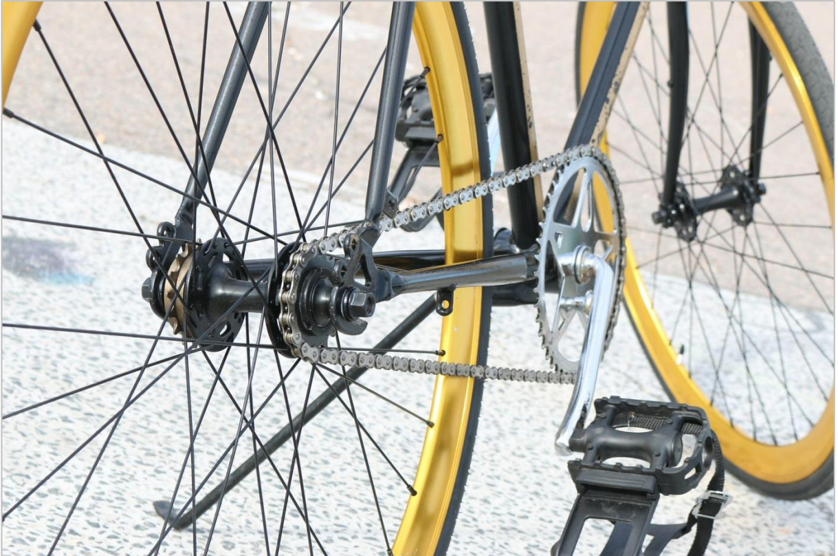
The chain and sprockets of a bicycle
